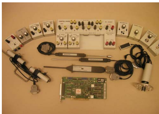
Inputs and outputs modules / sensors (in the front is the ADDA PCI card)
